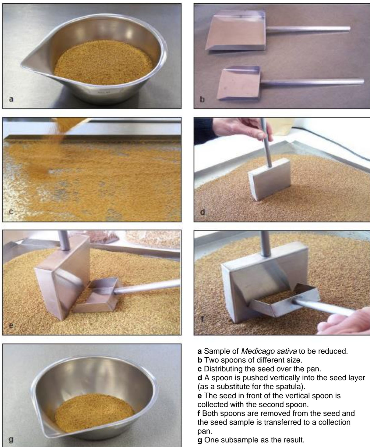
Figure 10: Sample reduction using the spoon method
